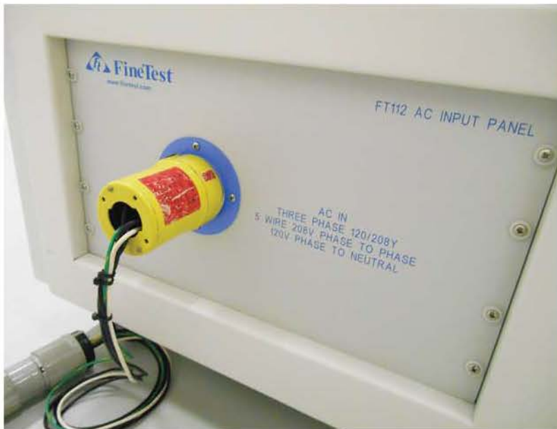
6U Custom Panel for AC Input
